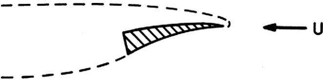
Figure 5.28 Supercavitating flow past a lifting foil with sharp leading edge.
